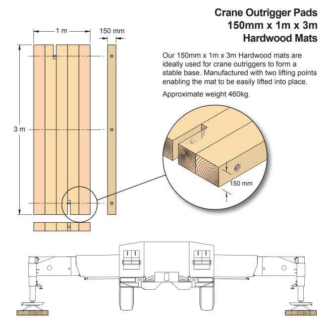
Usage of crane outrigger pads is the responsibility of the crane operator.
